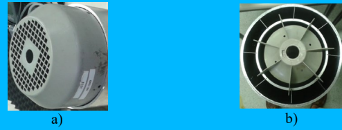
Fig. 11. Detail of the wind tunnel: a) fan cover, b) front view of the fan with the tunnel
