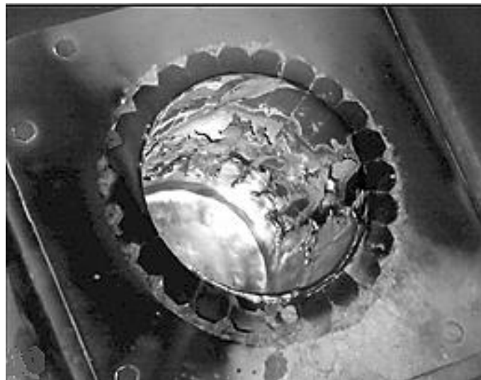
Figure 4-4. Deposits of Al and Mn on ISM crucible after melting TiAl; black ‘soot’ on the chamber and ‘flack’ deposits in the crucible [46]
