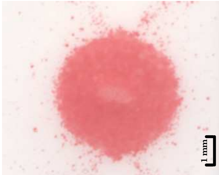
Figure 6.15: Patch of pressure measuring film scanned ( \delta_{\text{ref}} = 6 \text{ mm} and x = 1.1 \text{ mm} ).
