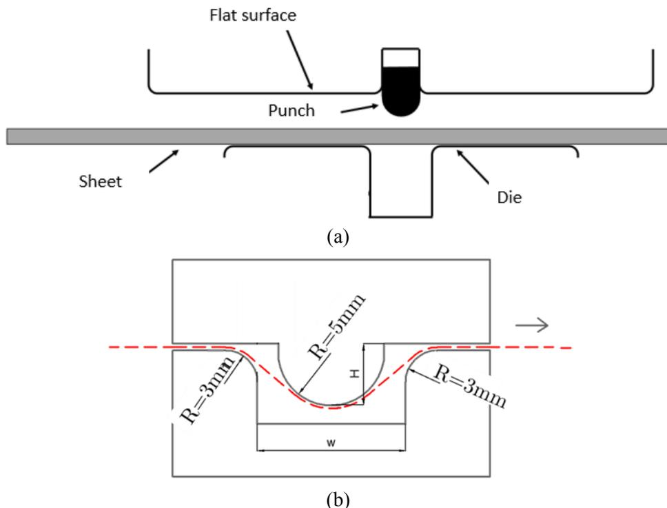
**Figure 1.** Drawbead simulations: a) Schematics of the drawbead and b) detail of the drawbead size.
