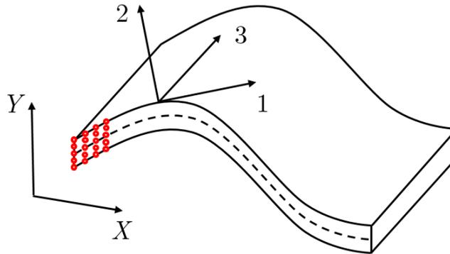
**Figure 4.** Sheet discretization for the internal bending moment evaluation.
