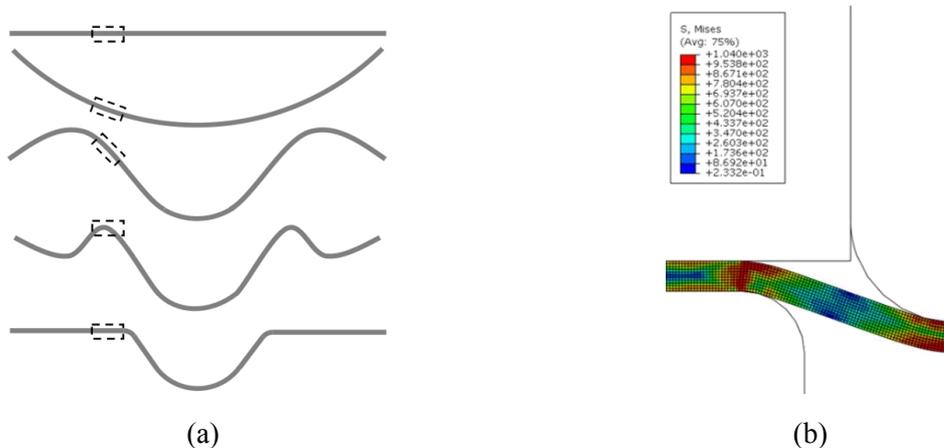
**Figure 2.** Numerical simulation result: a) shape of the sheet during the closure and b) stress distribution on the ‘curly’ area
