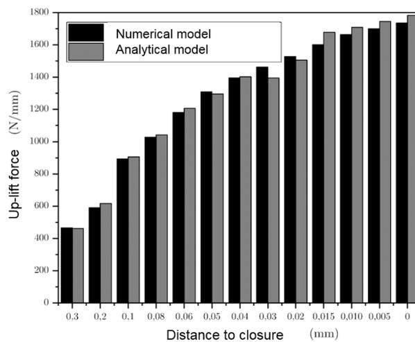
**Figure 5.** Comparison of the evolution of the up-lift force of the numerical model and the analytical model.
